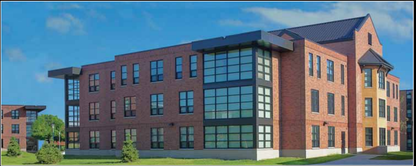
South Dakota State University – Brookings, South Dakota Special Blend; Thin Brick Precast; 1/2" x 2-1/4" x 7-5/8"; Wirecut Texture
